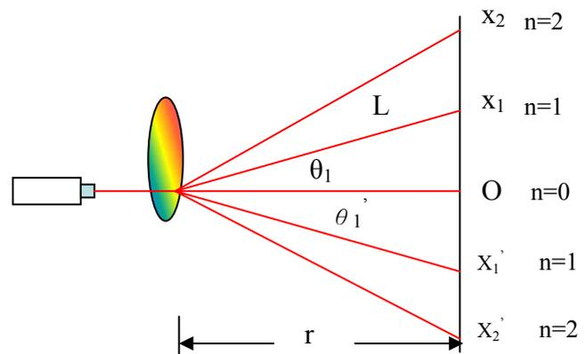
Fig. 6. Light pass through a transparent CD
