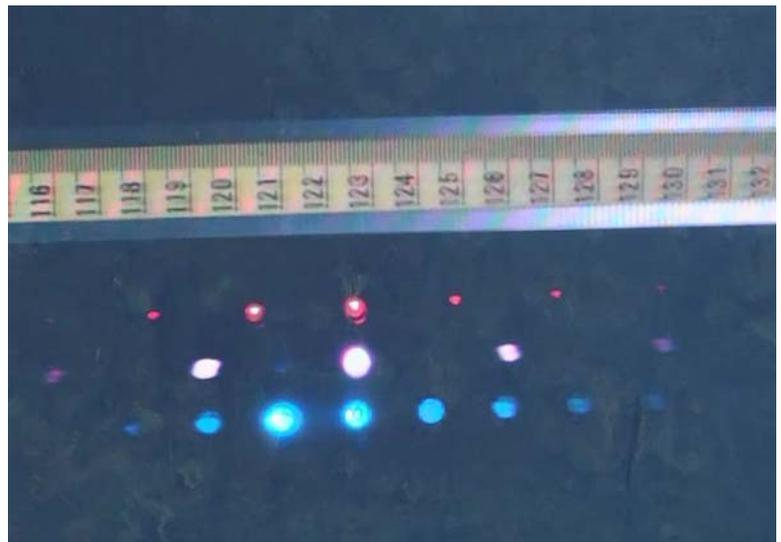
Fig. 16. Interference patterns of the red LED, IRED and blue LED
