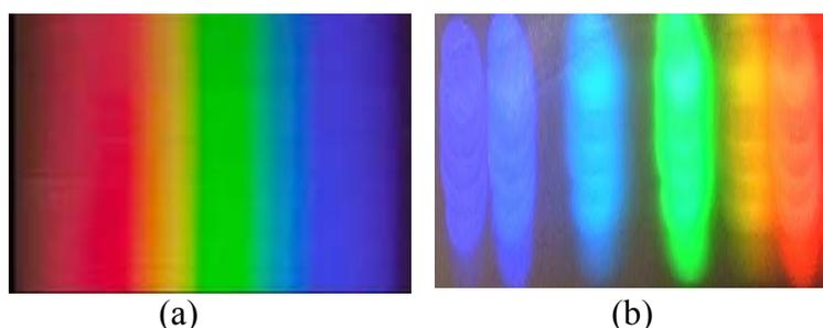
Fig. 8. Spectra of (a) 60W Incandescent bulb, (b) Phillips 15W compact fluorescent lamp.
