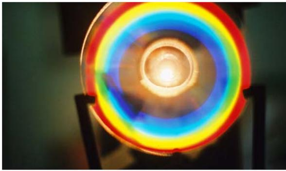
Fig. 12 Spectrum of a 60W incandescent bulb.
