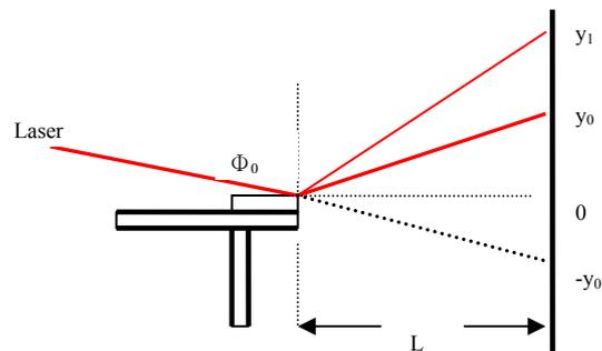
Fig. 9. Determine grating spacing of a CD
