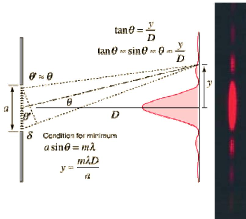
Fig. 3. Diffraction of a single narrow slit
