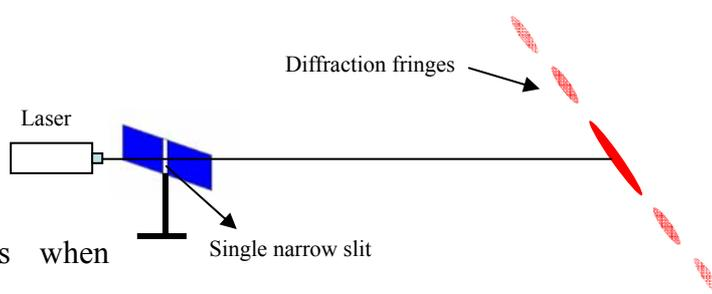
Fig. 1. Laser light diffraction by a single narrow slit.
