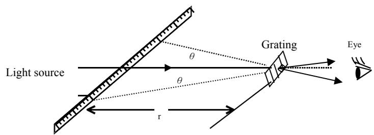
Fig. 5. Measurement of the wavelength of visible length
