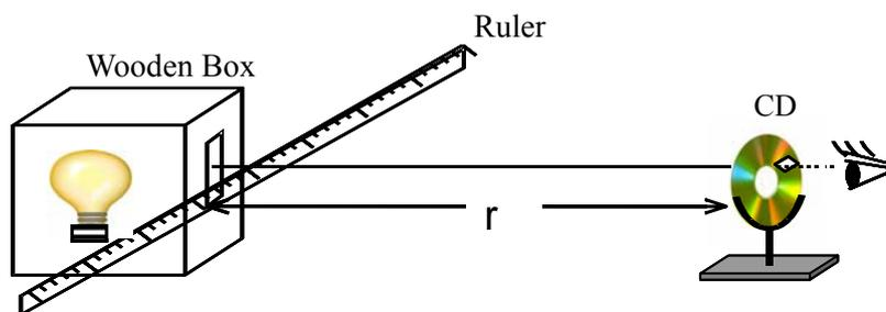
Fig. 7 Measure the wavelength of a lamp
