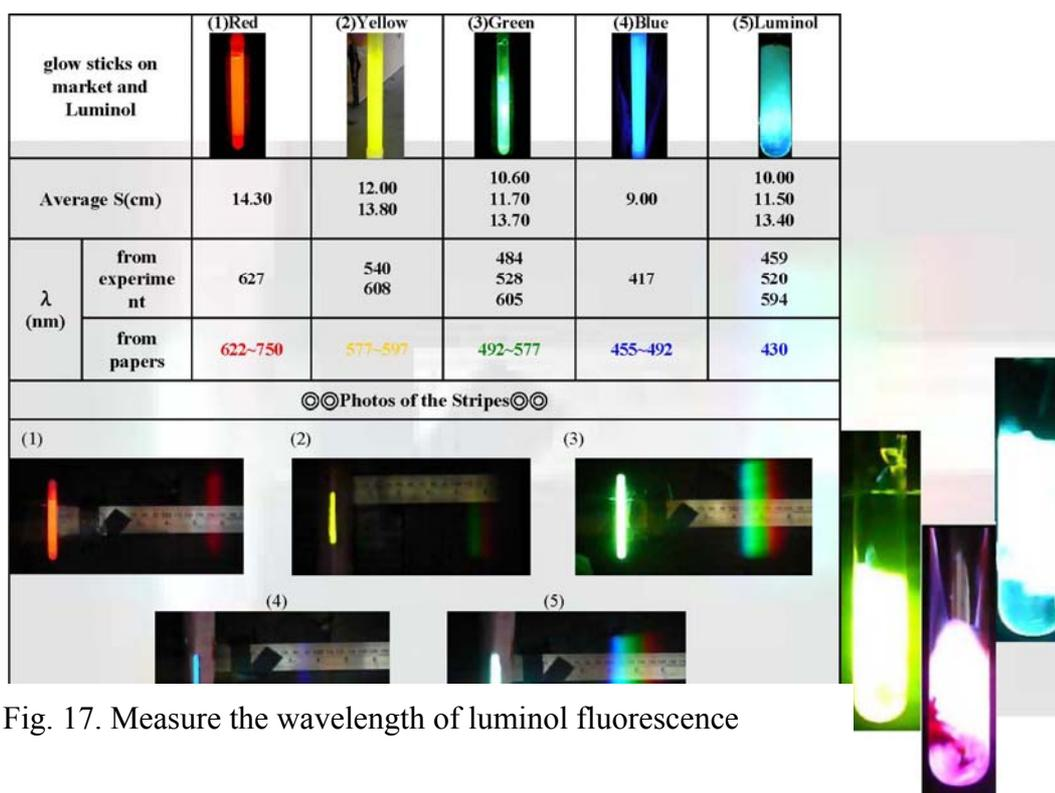
Fig. 17. Measure the wavelength of luminol fluorescence
