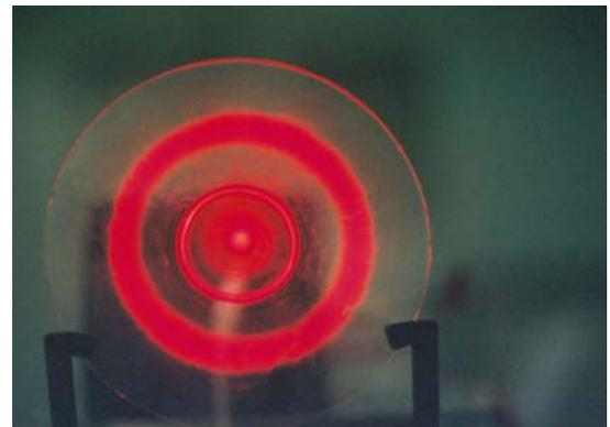
Fig. 15. Spectrum of a red LED
