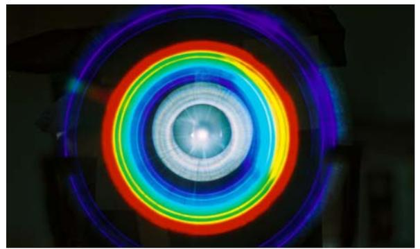
Fig. 13. Spectrum of a 15W compact fluorescent lamp.
